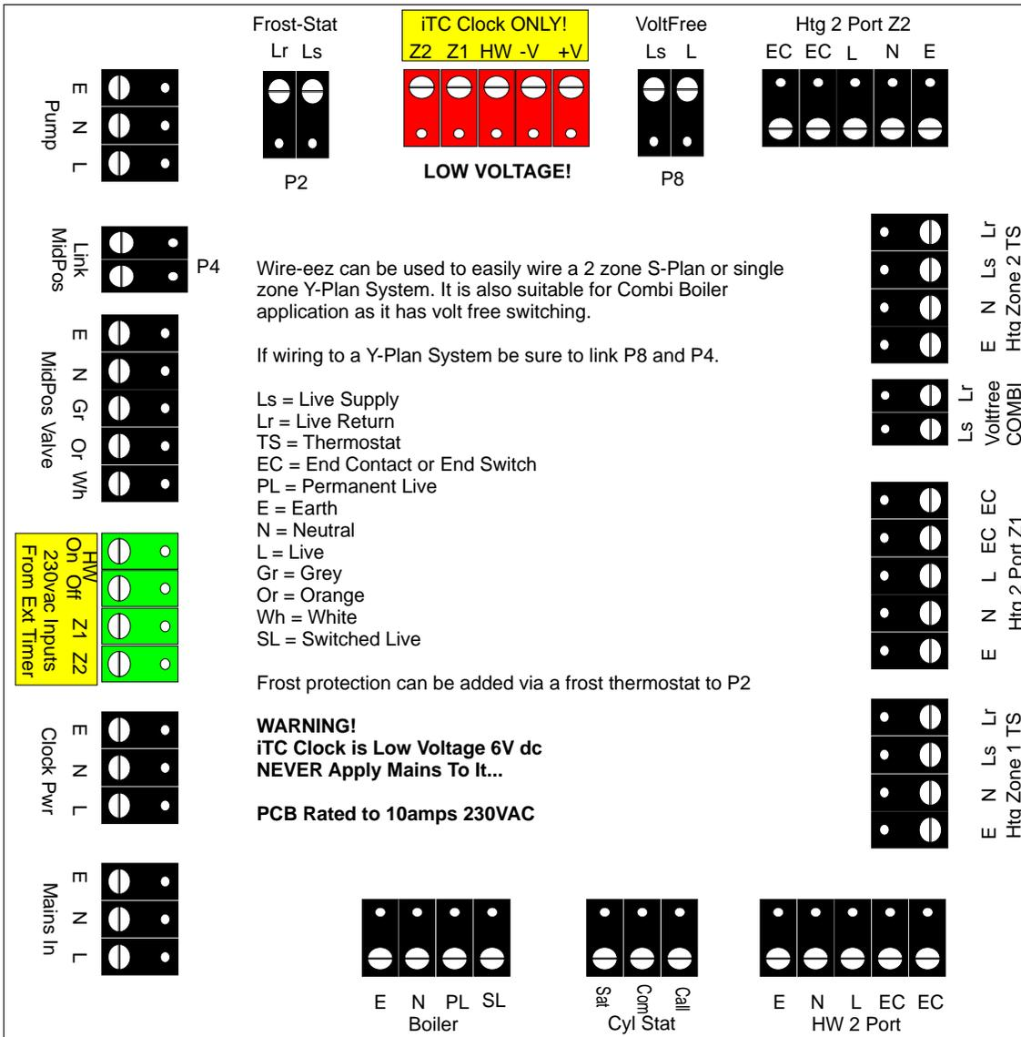
Wire-eez can make light work of wiring up to 2 heating and 1 hot water zone. It is best suited to S-Plan rather than Y-Plan and can be used with the iTC range of programmers and sensors or standard timers and room thermostats.
