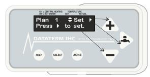
The Plus, Minus and Tap keys shown above also act as Up, Down and Right arrows, these are displayed on the screen when editing or setting plans and options. The position of the cursor is shown on the screen in the way of a flashing oblong.
